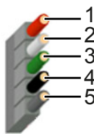
Fig. 5 Standard wire assignments 1x5 header connector female
